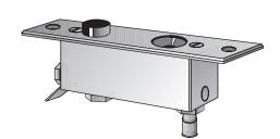
The standard version includes a 3 mm straight compressed air connector. If you need a swivelling angular connection, replace the "2" in the order number by "**WS**"
